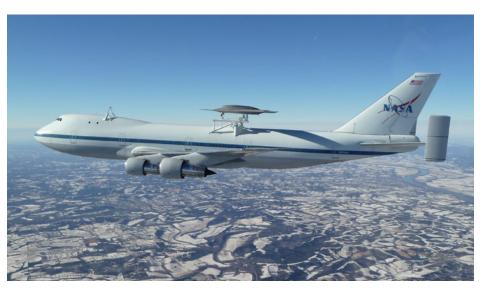
NASA's Shuttle Carrier Aircraft, a modified Boeing 747, carries Boeing's Phantom Ray during a test flight on Dec. 13 in St. Louis. Photo courtesy of NASA
