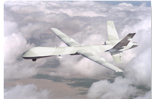
Predator B is powered by a turboprop engine and can carry a greatly increased payload.
